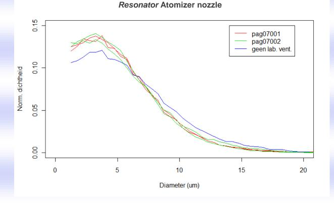
When supported by a ventilator, the spray is distributed more effectively over the surface area. Conclusion based on above droplet spectrum measurement with water and liquid: The Resonator atomiser with a spray capacity of 2 litres per hour still produces a very fine spray.
